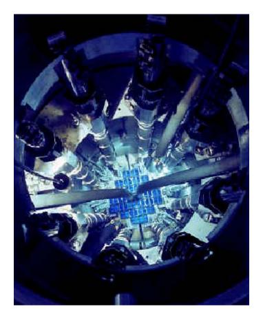
This is a view looking down into the reactor vessel into the core. The 28 fuel elements are seen at the bottom center of the picture. The twin tubes in the center of the core were used for irradiation of samples. Control rod drives are positioned around the periphery of the vessel, and are connected to right angle shaped control blades at the corners of the core. The bluish glow at the center is the Cerenkov radiatation All of the fuel elements were removed and shipped off site in 1997.
