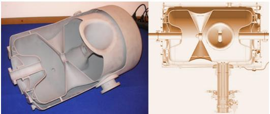
LEFT: A niobium double-spoke cavity surrounded by its titanium helium tank. RIGHT: 3D model of the integrated spoke cavity. PHOTO: Roger Ruber/Uppsala University | IMAGE: IPN Orsay
