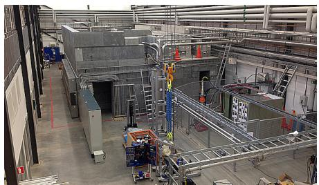
The FREIA Hall in Uppsala, Sweden. The bunker contains the facility's cryostat, and will house the ESS cryomodule prototype to be shipped from France later this year. Amplifiers for the testing will be set up in the foreground. PHOTO: Anders J. Johansson/Lund University
